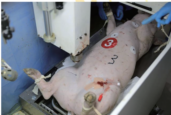
图 1 致伤前使动物右下肢外展外旋充分暴露于激波管口 Fig.1 Before injury, abduct and externally rotate the animal's right hind limb to fully expose it to the shock tube opening
